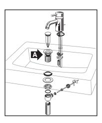
Mount the faucet and drain assembly (not included) on the sink following the manufacturer's instructions. Be certain to apply a bead of sealing putty on the underside of the drain (if required) (Part "A") in order to ensure a watertight seal between the sink and drain. Remove excess putty after installing drain on sink.
