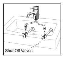
Connect supply line to faucet (finger tight) and carefully bend tubes to engage with the supply shut-off valves. Tighten connections at faucet and shut-off valves for secure seal.
