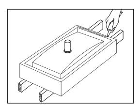
After checking fit and alignment, turn sink upside down and apply a generous portion of silicone adhesive around the under side of the rim near the edge. Place sink in position. Wipe off excess adhesive.
