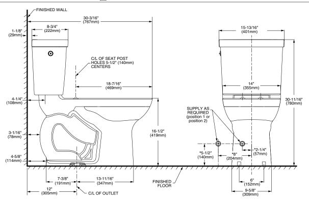
\* THIS COMBINATION IS DESIGNED TO ROUGH-IN AT A MINIMUM DIMENSION OF 305MM (12") FROM FINISHED WALL TO C/L OF OUTLET.
