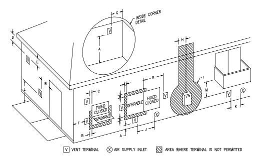
Figure 1 - Vent Terminal Clearances
