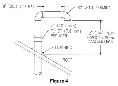
**NOTE:** For installations requiring both horizontal and vertical runs, the following rule must be followed: Total length of straight pipe (both horizontally and vertically) must not exceed the allowable length listed in the "Through The Wall" section of the table for total number of elbows used.
