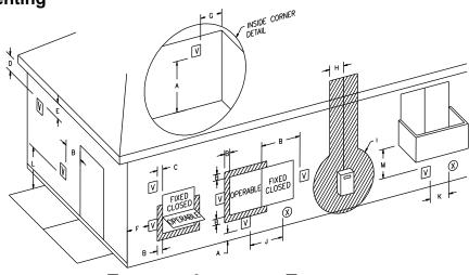
$\fbox$  vent terminal (X) air supply inlet  $\swarrow$  area where terminal is not permitted
