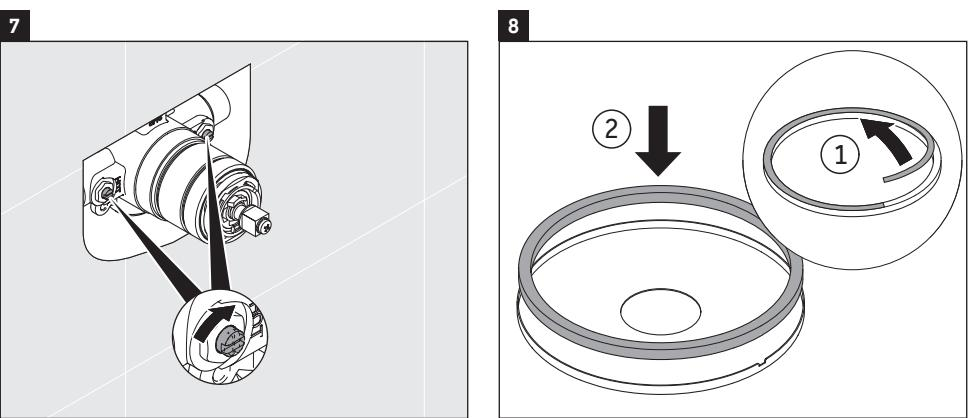
> Turn on hot and cold check valves by turning clockwise.
