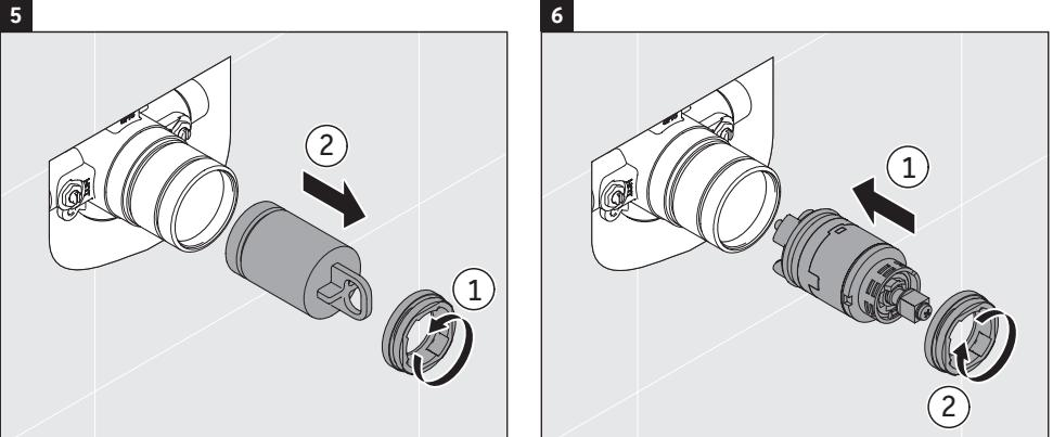
> Remove the handle protective cover by unscrewing the locking nut and removing.
