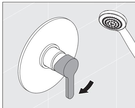
> Once handle testing is verified, turn handle on center to turn off.
