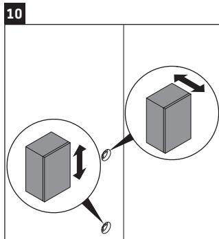
> Removing the plugs on the inside back wall of the cabinet will reveal screws which allow adjustment of the unit. The top screw will adjust front to back, and the bottom screw adjusts up and down.
