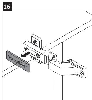
> Removing the plastic Duravit hinge cover will reveal three Phillips head screws.
