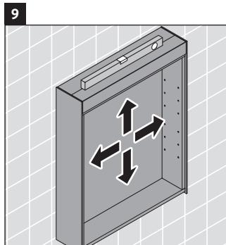
> Check the cabinet is leveled and securely attached to the wall.
