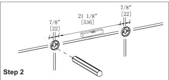
Position the backing plates flat side down on the wall and mark holes with pencil.
