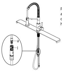
Push the quick connector (I) firmly upward and attach it to the receiving block (a). Pull down moderately to ensure the connection has been made.
