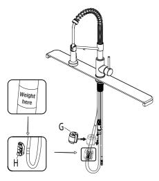
Install the weight clip (H) at the point of the hose marking "weight here". Insert the weight (G) onto the weight clip (H) by sliding it down onto the weight clip (H).
