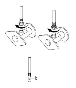
Attach waterlines to angle stops and tighten until snug. Turn on angles stops and check for leaks (DO NOT TURN FAUCET ON)
