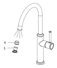
After installing faucet, remove aerator (4) with included aerator key (5). Turn water on for 30 seconds to remove any debris. Reassemble aerator (4).
