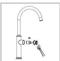
**Step 2:** Unscrew the locking nut with an adjustable wrench. Remove ceramic disc cartridge
