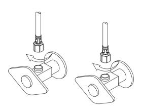
Attach waterlines(3) to angle stops and tighten until snug. Turn on angles stops and check for leaks (DO NOT TURN FAUCET ON)
