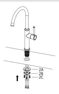
Insert faucet body (1) into hole in countertop. Install mounting hardware (2A, B, C) from underneath the countertop
