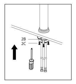
Adjust direction of faucet body (1) so that handle is on right side of faucet. Tighten mounting nut (2B) until snug. Tighten mounting screws (2C) to nut with Phillips screwdriver until snug
