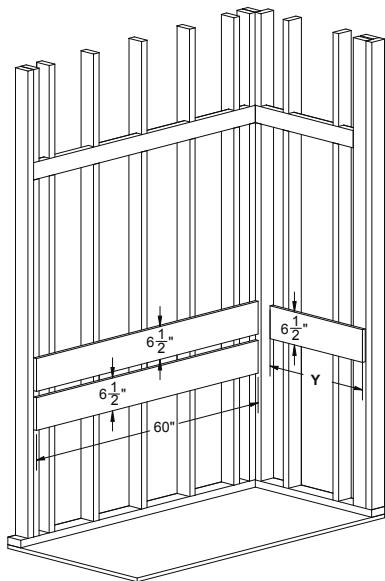
Additional bracing is required before grab bars are installed. Using  $\frac{3}{4}$ " plywood, reference the suggested measurements and attach bracing to the studs before final installation of the bathtub wall unit.
