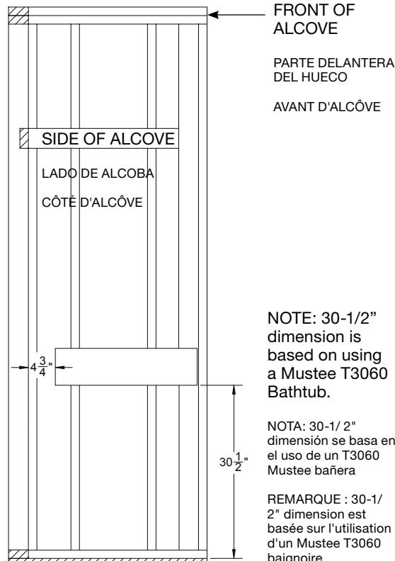
NOTE: 30-1/2" dimension is based on using a Mustee T3060 Bathtub.
